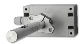
ADS-RH-D is a capacitive relative humidity (RH) sensor. It is equipped with an output relay with adjustable switching level and with analog 0-10V voltage / 0-20mA (4-20mA) current output. The measurement is performed periodically after about 8s. Based on these measurements it is possible to directly control the ventilation, air conditioning and heat recovery units.
